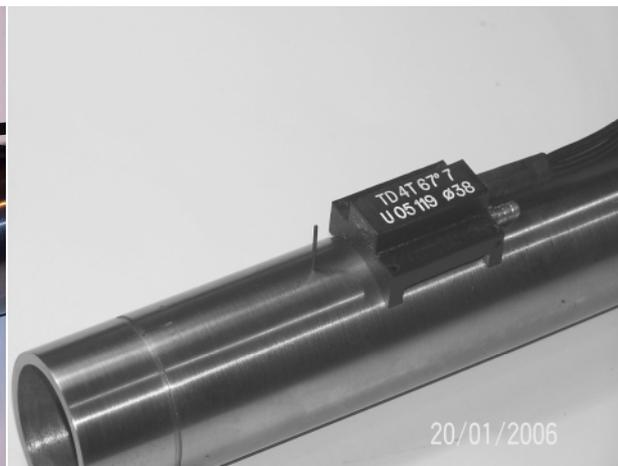
Fig.10 The profiled tandem probe in plastic casing (low profile)
