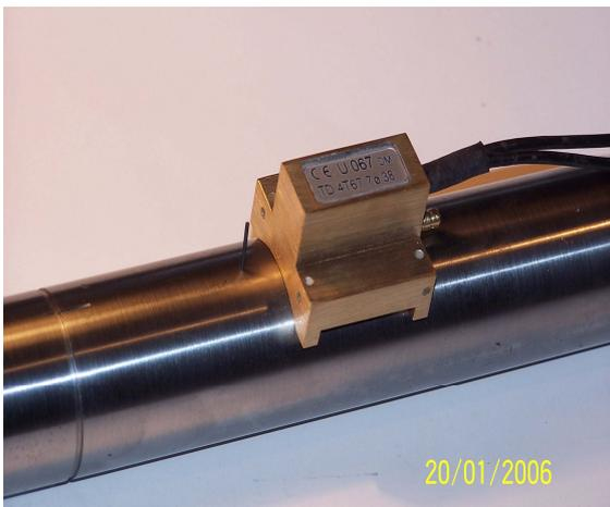
Fig.9 The profiled tandem probe in brass casing
