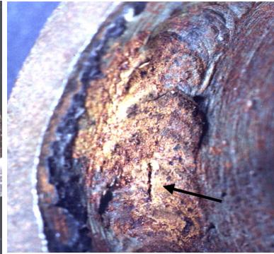
Fig.2 Circumferencial fracture in weld of pipe(Ø38, thick-3mm)
