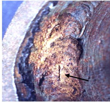
Fig.2 Circumferential fracture in weld of pipe(Ø38, thick-3mm)
